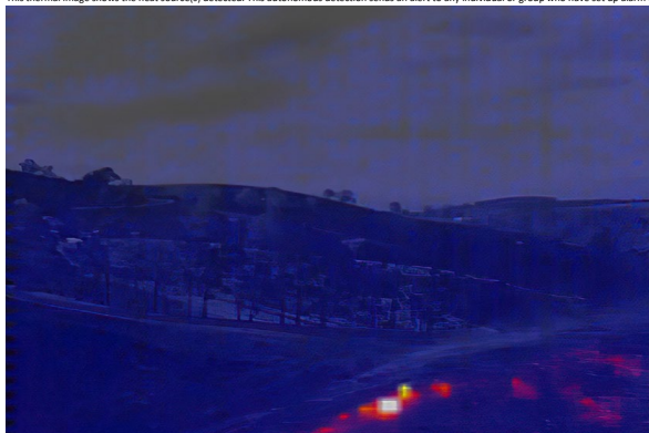
This thermal image shows the heat source(s) detected. This autonomous detection sends an alert to any individual or group who have set up alarm configurations
